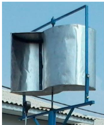
Fig. 5. Design 2; turbine Savonius H \neq 2D , D = 45 cm, H = 30 cm
