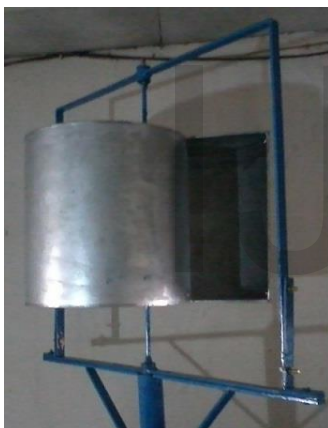
Fig. 4. Design 1 ; Turbine Savonius H \neq 2D , D = 45 cm, H = 30 cm
